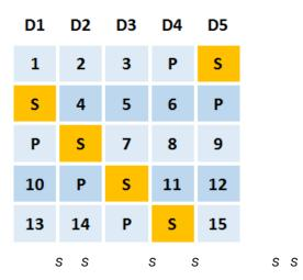
Assume that disk 2 has failed. RAID 5EE is under degraded mode.
