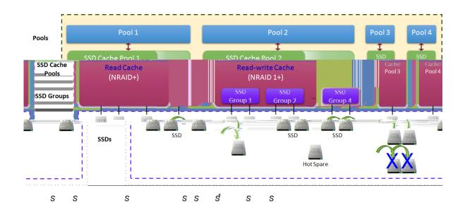
Take an example of SSD read cache; one or more SSDs with NRAID+ (which is described in the next section) are grouped into the "SSD Cache Pool 1" and assigned to the "Pool 1" for use. The maximum SSD quantity in an SSD cache pool is 8. When the SSD read cache is
