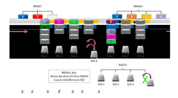
NRAID is a method of combining the free space on multiple disk drives to create a spanned capacity. A NRAID is generally a spanned volume only, as it can contain disk drives of various types and various sizes. RAID 0 consists of striping, without mirroring or parity. Adding a disk drive into RAID 0 needs to re-stripe the data. For SSD cache, it will have terrible performance when performing SSD cache and migrating RAID 0 at the same time. Let alone remove a disk drive.
