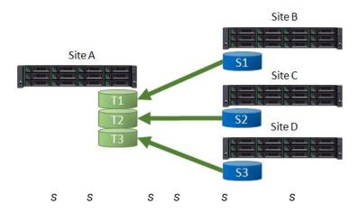
Multiple source systems replicate to a single target system. A Source Volume (S1) in Site B is replicating to a Target Volume (T1) in Site A. At the same time, a Source Volume (S2) in Site C is replicating to a Target Volume (T2) in Site A. So does S3 in Site D to T3 in Site A.
