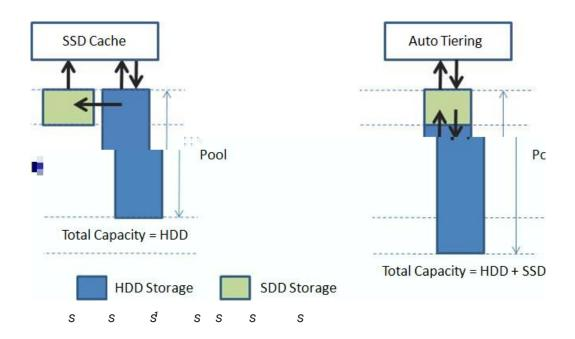
Total storage capacity in auto tiering is a sum of all individual tier capacities whereas in cache, the cache capacity does not add to the overall slower storage capacity. This is one of the key differences. In addition, SSD cache affects rapider than auto tiering because auto tiering will be affected by relocation the data in a period of time. So SSD cache warm-up timeframe is usually minutes/hours whereas tiering warm-up is usually in days.
