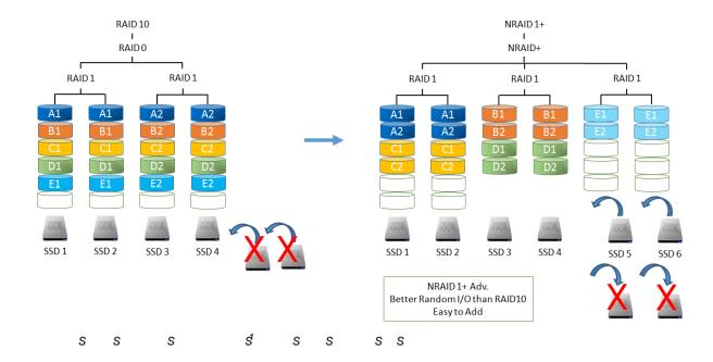
RAID 10 creates a striped set from a series of mirrored drives. The same, adding pair disk drives into RAID 10 needs to re-stripe the data. So it is hard to add SSDs into SSD cache pool.
