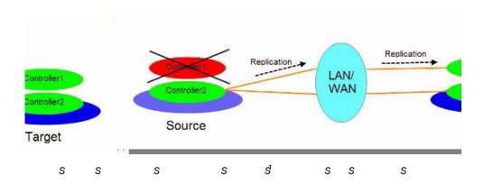
In another scenario, when controller1 fails on the target unit, the replication connection will be failed over to the second path from the controller 1 of the source unit to controller 2 of target unit.
