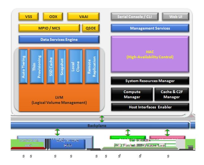
Base on LVM technology, it develops the features of auto tiering, thin provisioning, SSD cache and also data backup functions of snapshot, local clone, and remote replication. Upon LVM, QSOE (QSAN Storage Optimization Engine) which we are proud to develop, increases IOPS performance and overall system throughput. SANOS also supports several critical data services such as MPIO (Multi-Path I/O), MC/S (Multiple Connections per
