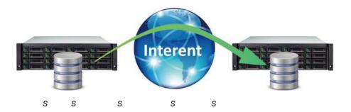
Remote replication uses the iSCSI function to set up a replication connection. It can use the full bandwidth of the assigned network port to allow the best backup speed. However, in order to balance replication traffic and non-replication traffic, the traffic shaping function can help to reserve necessary bandwidth for non-replication I/O.
