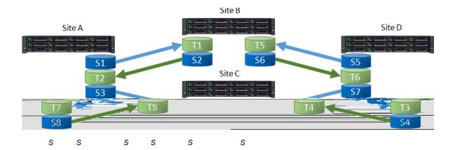
Combination with bi-Directional, one-to-many, and many-to-one, remote replication also supports Many-to-Many topology. Multiple source systems replicate to multiple target systems. A Source Volume (S1) in Site A is replicating to a Target Volume (T1) in Site B. At the same time, a Source Volume (S2) in Site B is replicating to a Target Volume (T2) in Site A. And does S3 to T3, S4 to T4, ..., S8 to T8.
