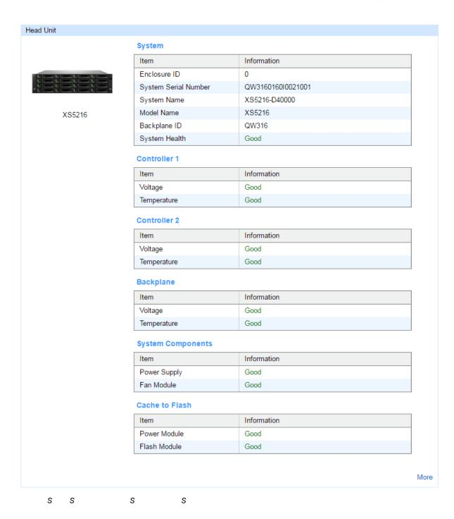
There are many voltage and temperature sensors on the controller and backplane. If the statuses of every sensor are Good, the information in this page displays Good. On the other hand, if anyone is not good, it will display Failed. So you may click More... to see details on what component has a fault.
