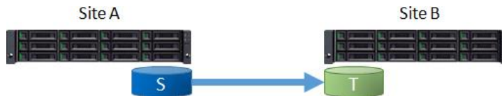
Figure 12-22 One-Directional Remote Replication
