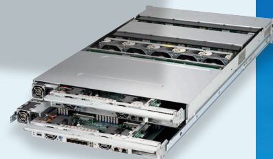
2U 40 Bay Dual Node Server with Dual Port All-Flash NVMe
