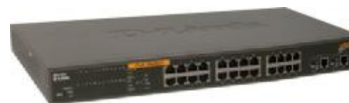
DES-1526 • 24 10/100M, 2 Combo Giga • PoE on all 24 ports • Smart Switch
