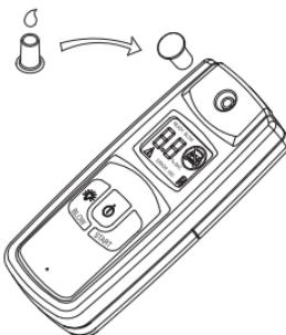
2. Power on the unit by pressing the “ON/OFF” key once, the unit will perform a self test procedure which takes approximately 12 – 18 seconds, indicated by counting down from 12 / 18 to 0 with flashing “READY” sign.
