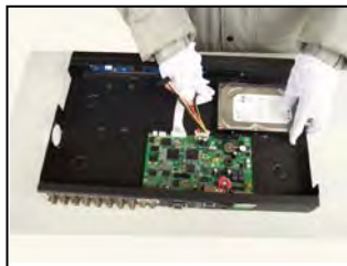
5. Install SATA power cables
