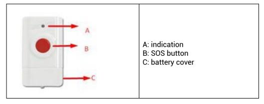
**Pairing:** switch the Sonix control panel to pairing mode, press the button on the SOS controller, the control panel will confirm the receipt of the code.
