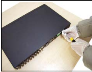
① disassemble the screw
