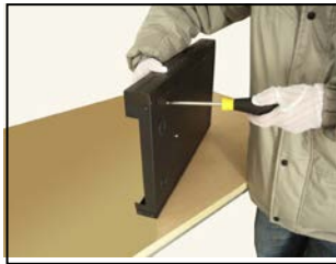
④ fix the screw of hard disk
