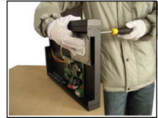
③ fix the screw of hard disk
