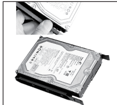
Put HDD bracket in the tool free
