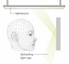
Unlike traditional curvedscreen CRTs (Fig 1), the innovative design of the MultiSync FE Series CRT deflects glare from overhead lighting, away from users, for a more comfortable and productive viewing experience (Fig 2).
