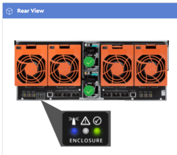
Figure 58: Identification LEDs Enabled
