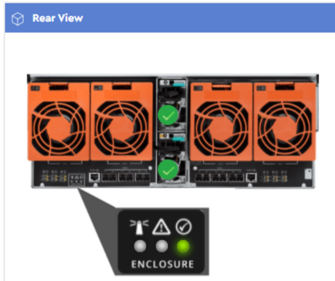
Figure 59: Identification LEDs Disabled
