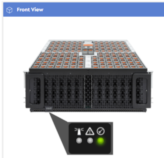
Figure 53: Identification LEDs Disabled
